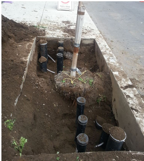
Fig. 1 The layout of lysimeters installed in a tree pit
